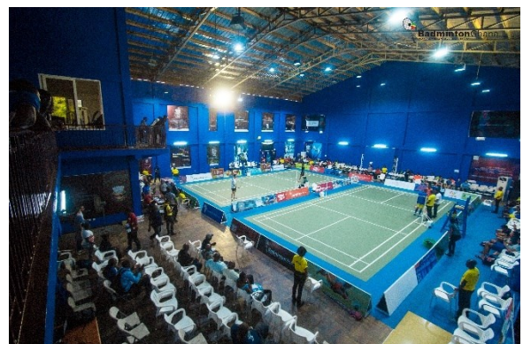
Sports hall structure, lights and division netting must be aligned between badminton courts.
